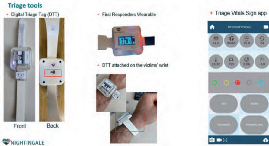
Figure 3. Triage tools, including the DTT, First Responders Wearable - FRW (similar device with monitor) and the Triage Vital Sign App (TSVA), which manages the DTT.
