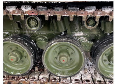
Fig. 4. Tank chain during disinfection © V. Steudel
