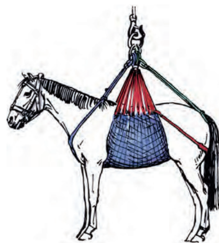
Figure 4: The Animal Rescue Transportation Sling in correct position (Source: M. Haab – Vetsuisse Zürich)
