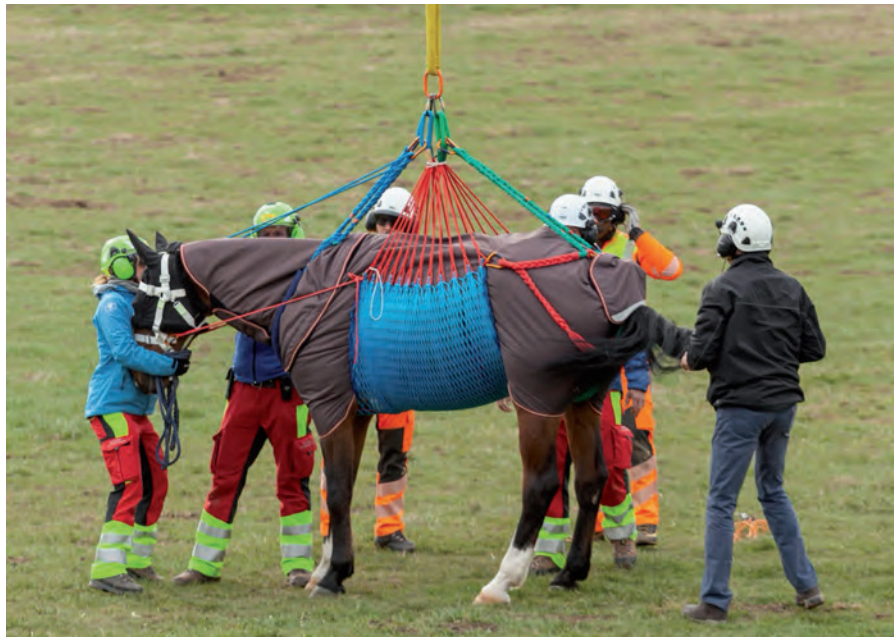
Figure 6: The complete flight equipment, which consist of a flight bonnet, the flight halter, the ARTS Sling and the blanket (Source: Department für Pferdechirurgie – Vetsuisse Zürich)
